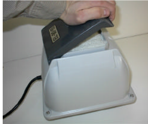
B. Remove the filter cover (1) from the overall cover (3).
