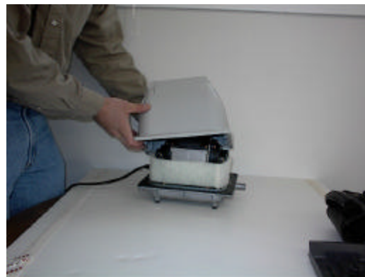
B. Remove the overall cover (3).
