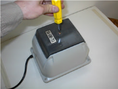
A. Remove screw (31) from the filter cover.
