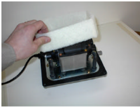
C. Remove sound attenuating material (4).
