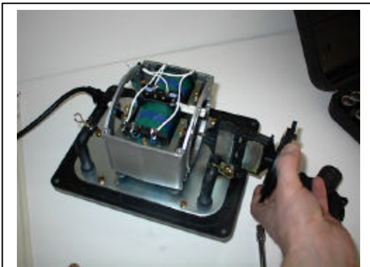
B. Remove the diaphragm holder (10) and the magnet (9) after opposite diaphragm holder (10) has been removed.
